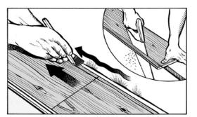
Put the first plank in the next row in place. Take the next plank. Place it on the subfloor and push it into the long side joint. Angle the plank a little bit so the tongue enters the groove. Slide the plank in place over the end joint and press it firmly down.
