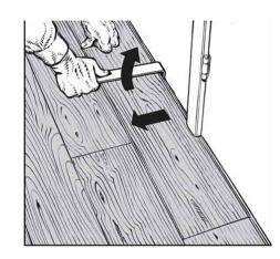
To calculate the correct width of the last row. Place a full row of tiles directly on top of the last installed row of full tiles. Use the full width of a scrap piece of tile. Place the tongue side against the wall and the pencil against the extended groove and mark a line the length of the wall. Cut along the pencil line.
