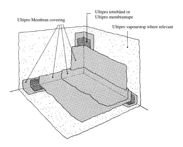
Note. When the Ultipro Vapourmat is required, it is installed between the two layers of Ultipro Membran.
