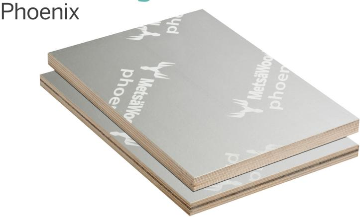
Metsä Wood Phoenix plywood products provide enhanced fire performance for uses in tranport industry. The product range consists of birch plywood and Sonex Light sound-absorbing sandwich panels overlaid with a special aluminium overlay. Phoenix products meet the requirements of many demanding end use applications.
