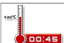
10. Allow the adhesive to cure to the specified time prior to applying any load or torque. Do not move or load the anchor until it is fully cured (attend Annex B 6).
