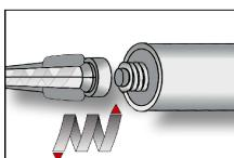
3. Attach the supplied static-mixing nozzle to the cartridge and load the cartridge into the correct dispensing tool. Cut off the foil tube clip before use. For every working interruption longer than the recommended working time (Annex B 6) as well as for new cartridges, a new static-mixer shall be used.
