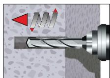
1. Drill with hammer drill a hole into the base material to the size and embedment depth required by the selected anchor (Table B1, B2, or B3), with hammer (HD), hollow (HDB) or compressed air (CD) drilling. The use of a hollow drill bit is only in combination with a sufficient vacuum permitted.
