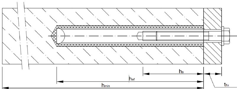
$t_{fix}$  = thickness of fixture
