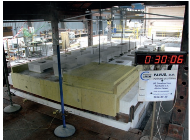
Figure 10. Sample after 30 minutes - fire protection system ISOVER FireProtect® fulfils its function for 100 %, roof is without any deformation (bending stress, the same as would be under cold conditions)
