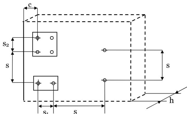
**fischer long shaft fixing FUR****Annex 7****Minimum distances and dimensions in masonry**
