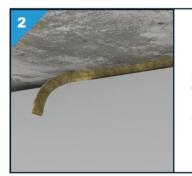
If backing is applied, cut it slightly wider than the joint width and make sure that it is applied to the correct depth in the joint.
