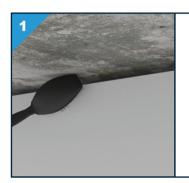
Make sure the joint is free from dust, dirt and grease. Moisten the structure, if necessary.
