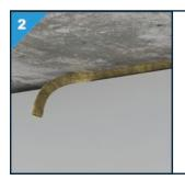
If backing is applied, cut it slightly wider than the joint width and make sure that it is applied to the correct depth in the joint.
