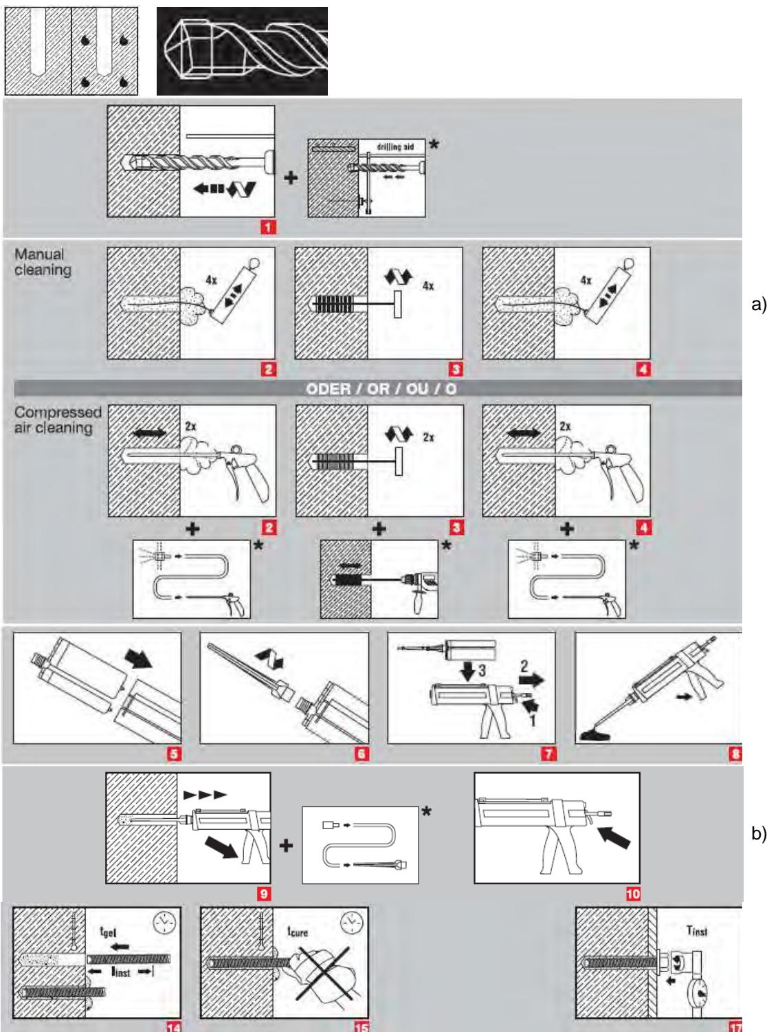
**a)** Note: Manual cleaning for element sizes  $d \leq 16\text{mm}$  and embedment depth  $h_{ef} \leq 10 d$  only!
