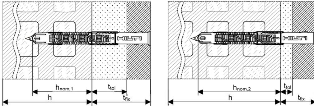
Intended use in precast prestressed hollow core slabs ( $w/e \leq 4,2$ )
