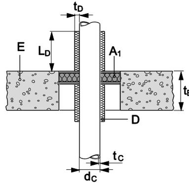
**Steel pipes (C) with continued insulation (D) – interrupted**
