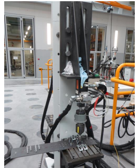
Test setup for cyclic tension tests
