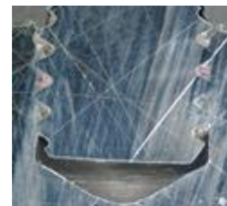
Fastening mechanism of the S-BT stud in steel
