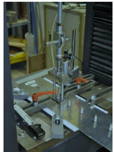
Test set up for tension tests
