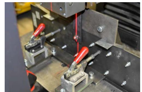
Test set up for shear load testing
