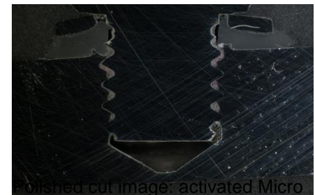
Micro encapsulation on the tapping thread of the S-BT fastener
