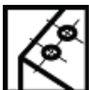
Small edge distance and spacing
