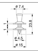
Powder-actuated fastener and fastening tool:
