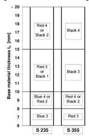
Note for S 275: Start with recommendation for S 355. In case of too much energy: Reduction of tool energy setting or change of cartridge colour till correct stand-offs  $h_{\text{NVS}}$  are achieved.
