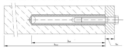
$t_{fix}$  = thickness of fixture
