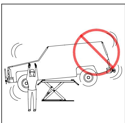
Lifting a vehicle with the engine running is prohibited.
