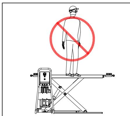
It is forbidden to climb aboard the vehicle both during the movement stages and when the vehicle is being lifted.
