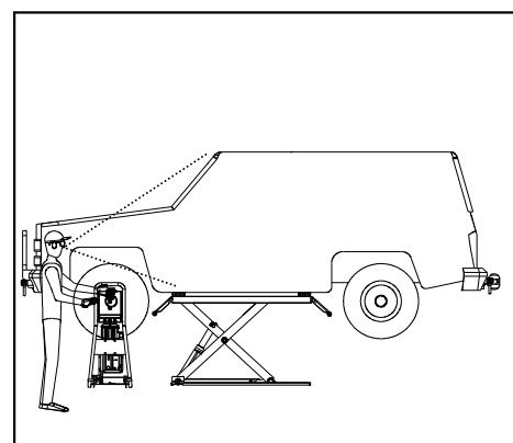
The vehicle to be lifted must be placed on the lift as illustrated in the load distribution diagram.
