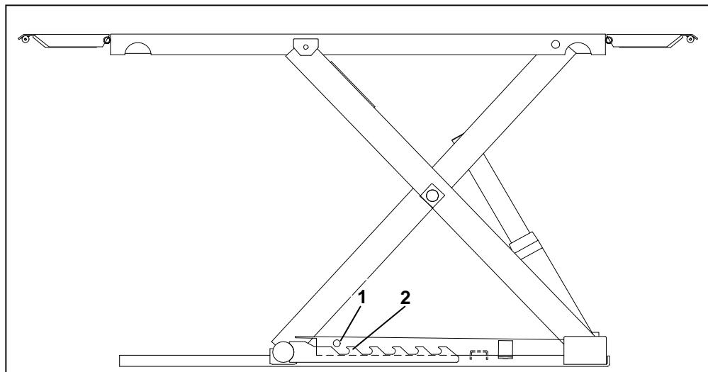
**Everyday, before using the lift, check that the mechanical safety device functions correctly: to this end check the pin of each of the two moving brackets (1) is correctly inserted into the corresponding fixed teething (2) when the control button is released.**
