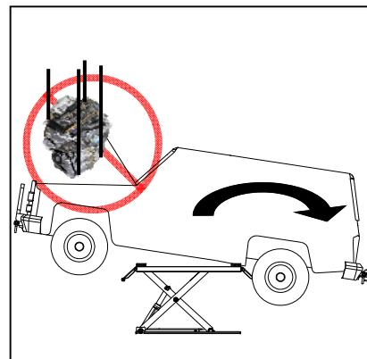
Before lifting or lowering, it is compulsory to check the stability of the system of the vehicle's lift.
