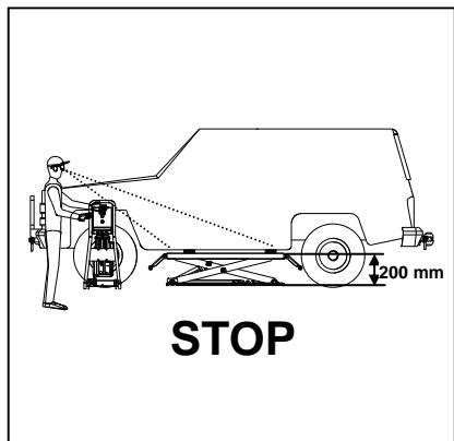
Before entering the working area, it is compulsory to turn the lift off setting the locking switch to "OFF - 0".
