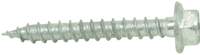
1192 4.. Fasthetsklasse 8.8 ISO 898/1 Rm = 800 N/mm2 Rp0.2 = 640 N/mm2 Varmforsinket 50 - 80 µm
