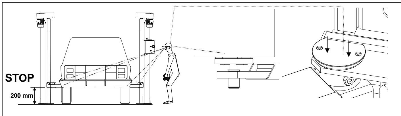
Before entering the working area, it is compulsory to turn the lift off setting the locking switch to "OFF - 0".
