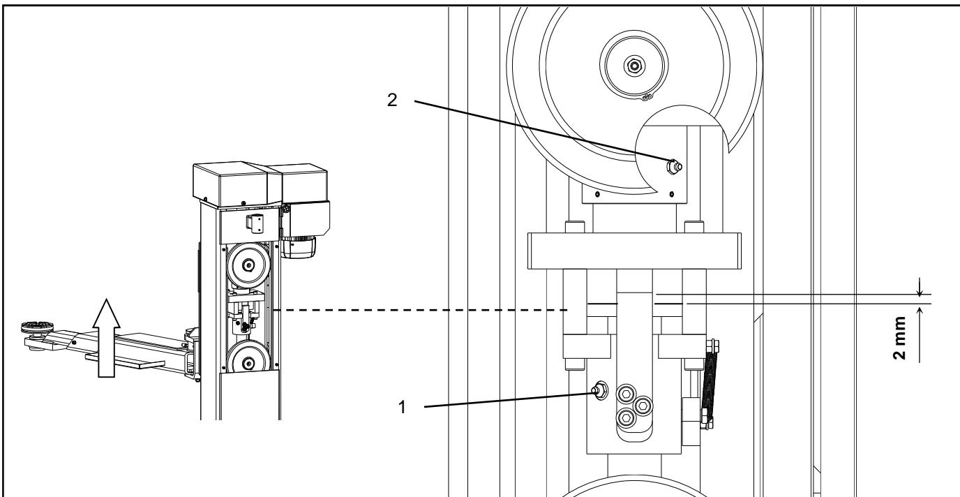
For both columns: remove the casings (1) installed at the top of the column and inject all-purpose grease in the specific grease nipples (2) on the transmission screw support flange, below the pulley.
