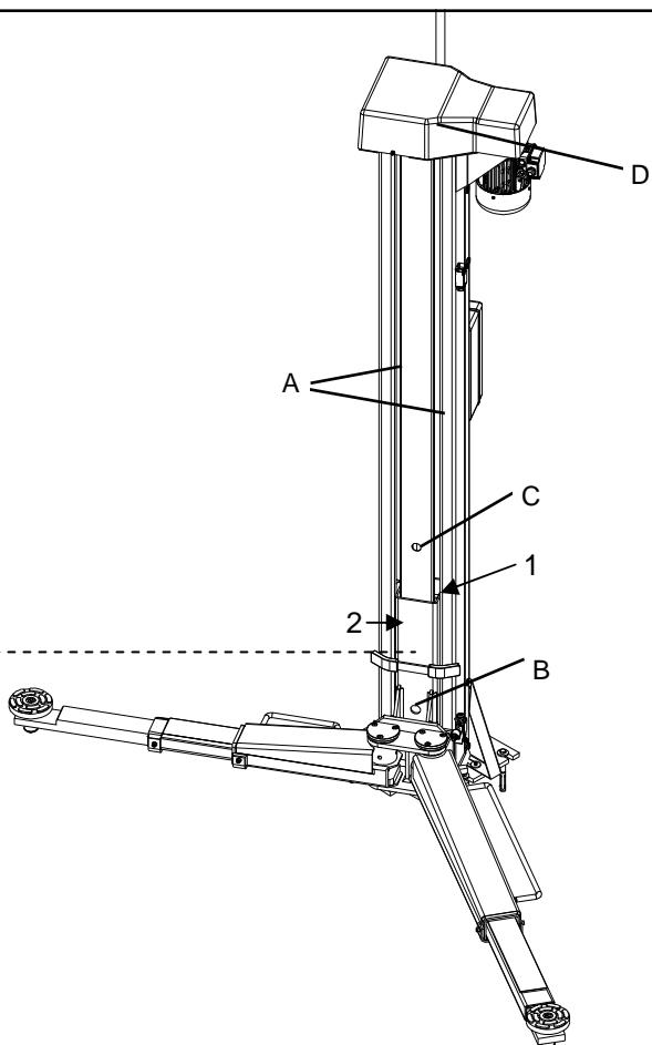
For both columns: grease the safety leadnuts (3) through the specific grease nipples. It is unnecessary to remove the column protection casing to do this: stop the carriages when the hole provided in the carriages (B) align with the hole present in the casings (C) so that it is easy to access the grease nipple.
