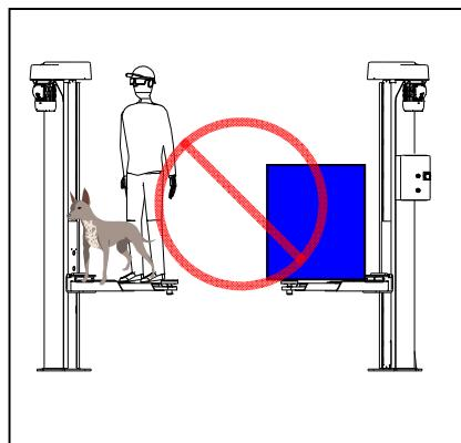
It is forbidden to climb aboard the vehicle both during the movement stages and when the vehicle is being lifted.
