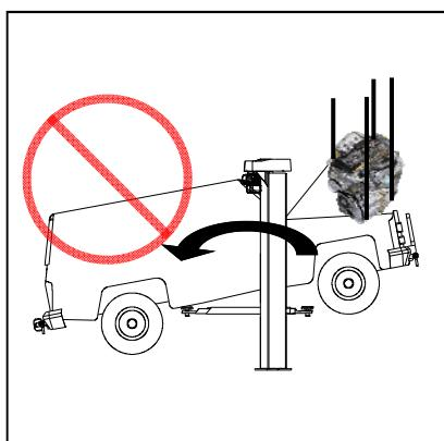
Before lowering, ensure that there are no objects and/or obstacles that could interfere with the movement in the area below the vehicle, the lifting arms and the trucks.
