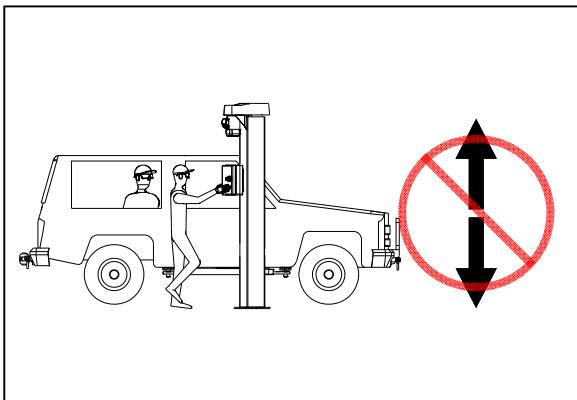
In the event of irregular or anomalous sounds, it is compulsory to stop all operations immediately and find the cause of the anomaly. If in doubt, avoid any improper operations and contact the technical service centre.
