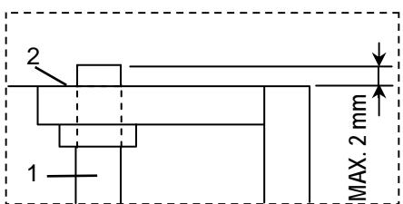
When the rod (1) is over the trolley (2) more than 2 mm: plan replacing the load bearing nut
