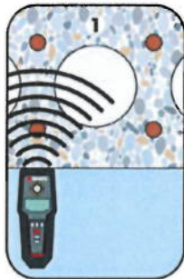
Locate the prestressing steel
