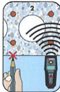
Mark the prestressing steel and locate the second prestressing steel
