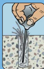
Clean drilled hole
