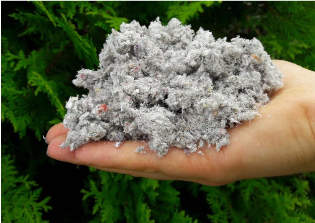
Figure 1: Loose fill cellulose insulation material
