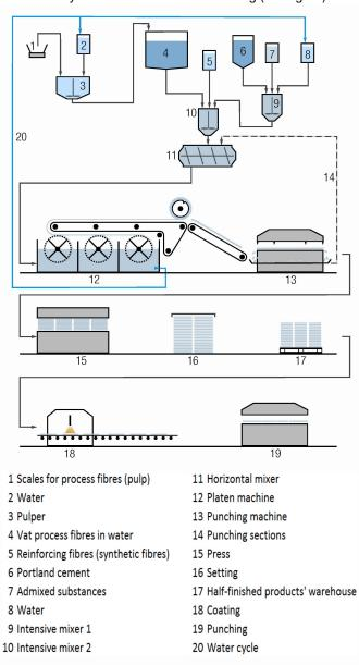
The raw materials are treated with water to a homogeneous mixture. The mixture is pumped into head boxes, in which sieve cylinders rotate, that are dewatered inside. Thereby the sieve surface is covered with a thin fleece of fibre cement, which is transferred to the endless circulating conveyor belt (transport
