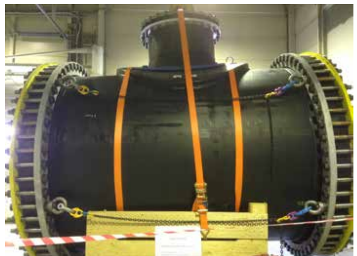
Picture 3 - Full scale pressure test of OD1000 saddle on OD2500 pipe to 2 bar
