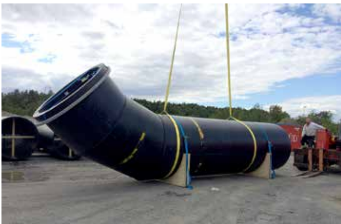
Picture 6 - OD2100 mm SDR26 bend
