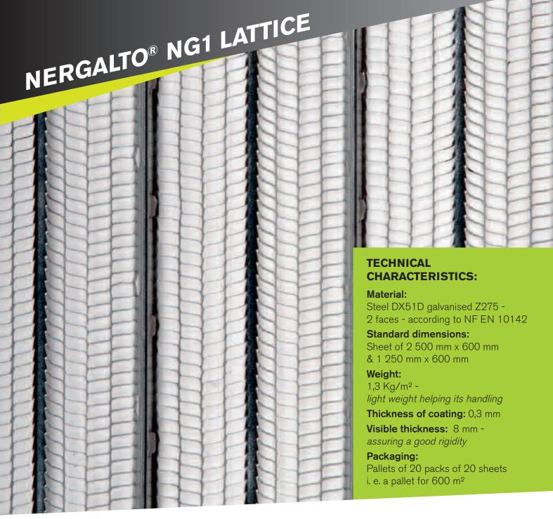
A real reinforcement, the NERGALTO NG1 lattice gives resistance and support to your renders both on the interior and exterior:
