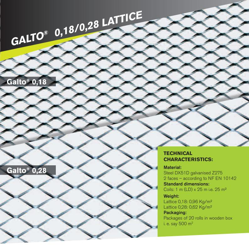
For hydraulic lime plasters or renders, METAL DEPLOYE proposes a specific solution with GALTO®, the non ribbed metallic lattice. It is generally applied to continuous elements (wood, masonry...) and increases the adhesion of hydraulic renders to the supporting element and limits the risks of cracking and micro cracking.
