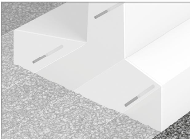
Fig. 15: Schöck Dorn: Expansion joint in cantilevered wall
