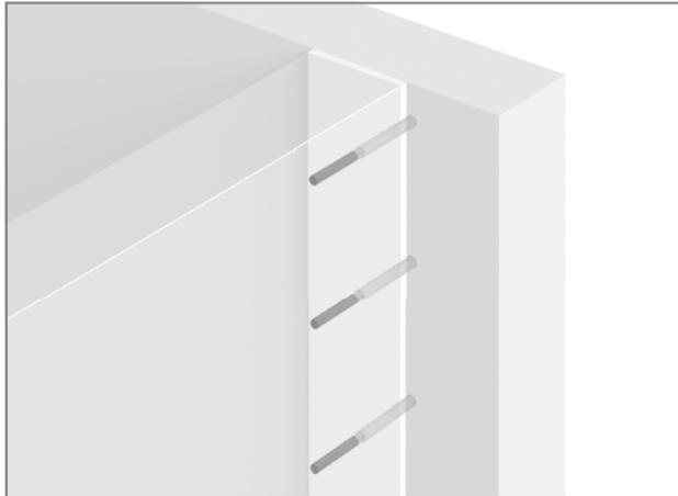
Fig. 11: Schöck Dorn: Connection wall-wall (face-flank)
