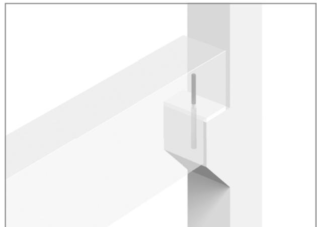
Fig. 16: Schöck Dorn: Position security of a beam on a corbel
