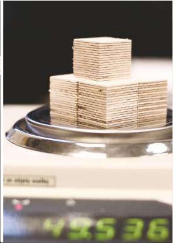
▲ **Figure 2.6. Weighing of plywood samples, to determine their moisture content and density**
