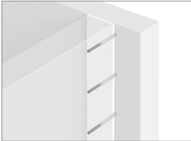
Fig. 11: Schöck Dorn: Connection wall-wall (face-flank)
