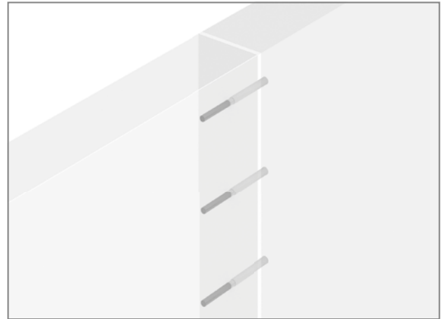
Fig. 12: Schöck Dorn: Connection wall-wall (face-face)
